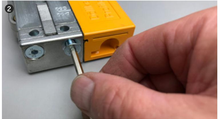
3 The blade must always be up to stop are inserted. Tighten the blade clamping plate.
