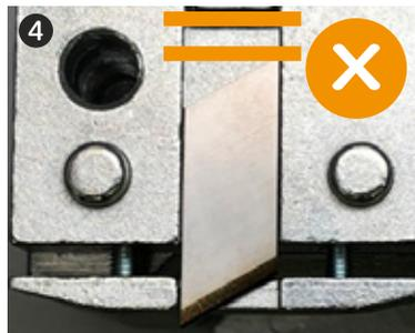
5 FALSE: turn the blade. Blade breakage!
